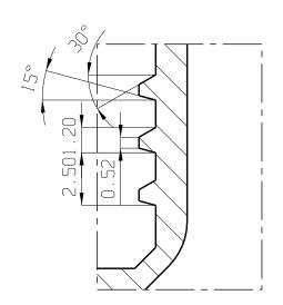
PITCH OF THE THREAD = 10 mm 4 START THREAD ANGULAR DEVELOP = 180° Date
